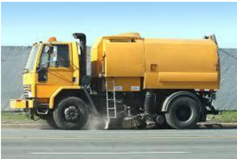
Figure 5.4 – Typical Road Sweeper
